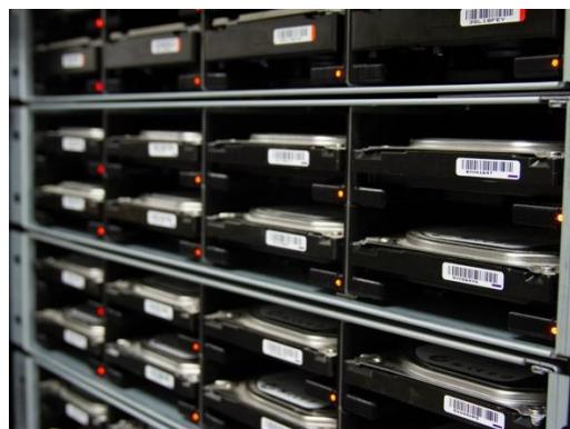
During the initial testing phases, the software scans for critical issues, such as helium gas leaks in modern helium-filled drives. This early detection allows stopping the testing as soon as possible, which reduces the overall time required for testing. Consequently, it improves the efficiency of the testing process.
